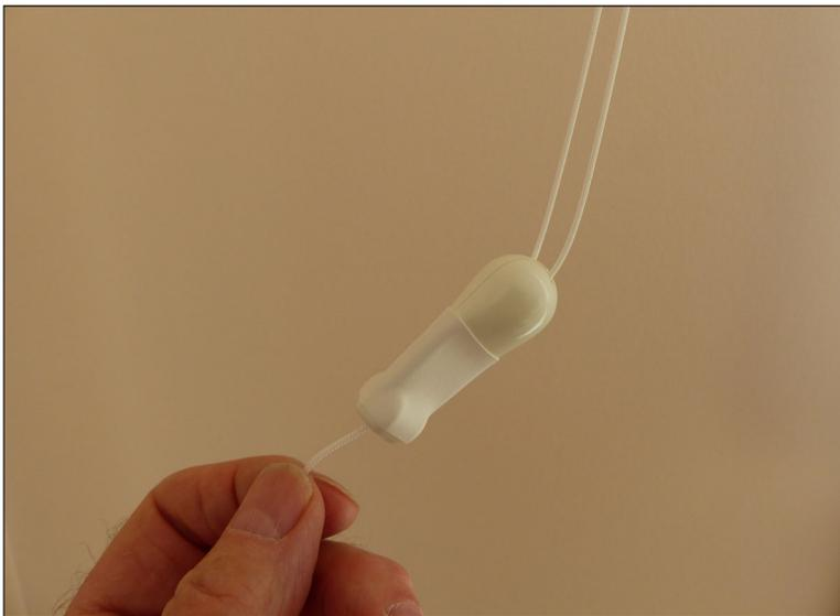
8. Finished. The connector is tightly encased in the tubing and will not split open, even when the pull-knob is jerked hard. If a connector needs to be opened later, the shrunk tubing comes off cleanly when slit.
