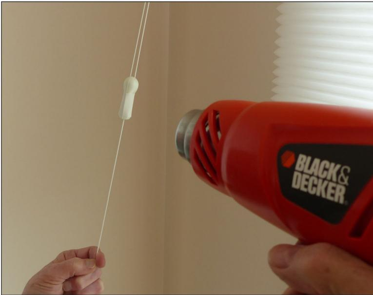
7. I have used a match or lighter to heat up tubing of this type when applied to wiring, but for this job I needed gentler heating to avoid damaging the connector or the cords. So I used an inexpensive Black & Decker 1375-watt heat gun to shrink the tubing around the connector.
