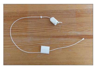
2. Slip a tubing segment over the end of the lower cord. (I had to do it this way, opening the connector and freeing the cord end, because the tubing segment was too narrow to fit over the pull-knob. Larger tubing would have fit over, but it would not have shrunk enough to do the job.)
