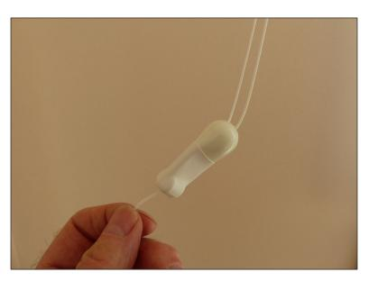
8. Finished. The connector is tightly encased in the tubing and will not split open, even when the pull-knob is jerked hard. If a connector needs to be opened later, the shrunk tubing comes off cleanly when slit.
