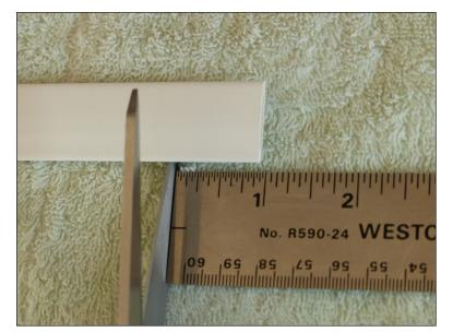
I bought one strip of tubing and cut 18 one-inch segments to slip around the connectors on the nine new shades. (Since these were top-down/bottom-up shades, there were two connectors per shade). Lots of tubing was left over to re-apply if any connectors needed to be opened, which required that the tubing be cut free.
