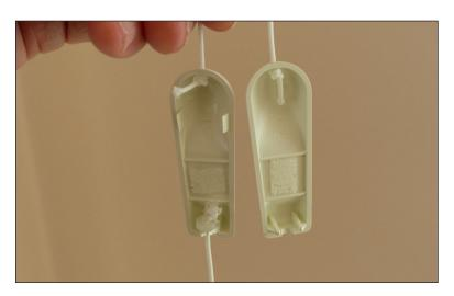
1. Pop the connector apart. Remove the single lower cord coming out between the two parts. There is no need to untie the knot by the plastic washer. Just pull the cord out of its slot.
