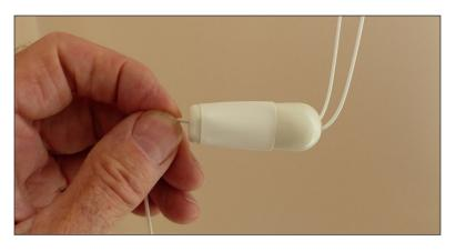
6. The fit should be fairly tight, even before heat is applied to shrink the tubing.
