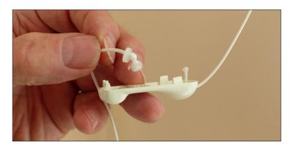
3. Place the single cord back into the connector, washer on the inside, and reassemble the two halves. Take care that the cut ends of the cords are not caught between the halves, or the connector won't close properly.
